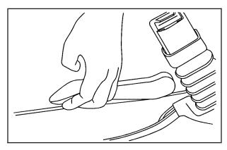
To adjust the seatback, lift the front of the lever located on the inboard side of the seat cushion.
